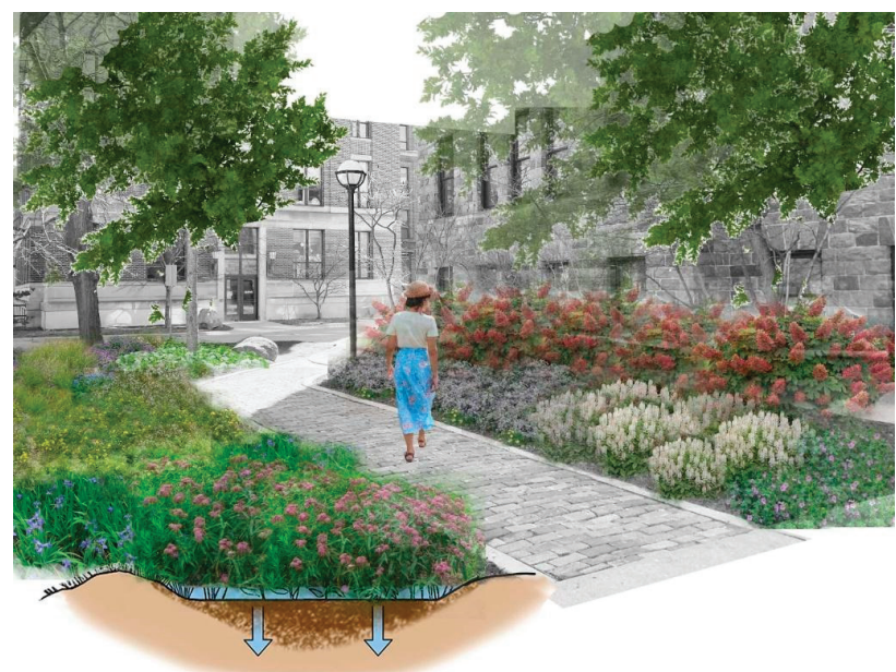
Figure 8. Visual to illustrate application of Typology 3 and Typology 4 in an urban setting, where it provides multifunctional benefits of pollinator habitat, improved water infiltration (shown as arrows), and aesthetic enjoyment.
