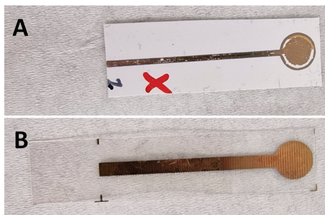
Figure 5. Examples of the initial batch of PET-based (A) and PEN-based (B) samples. Red “x” indicated samples that delaminated sections.
