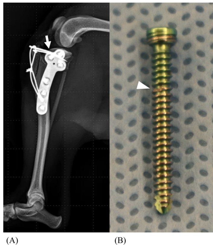
Figure 5. Mediolateral radiograph of the proximal pin group (A). During pin insertion, the pin bends due to the limited space caused by the proximal tibial plateau segment locking screw (arrow). The photograph of the damaged proximal locking screw due to K-wire insertion (B).
