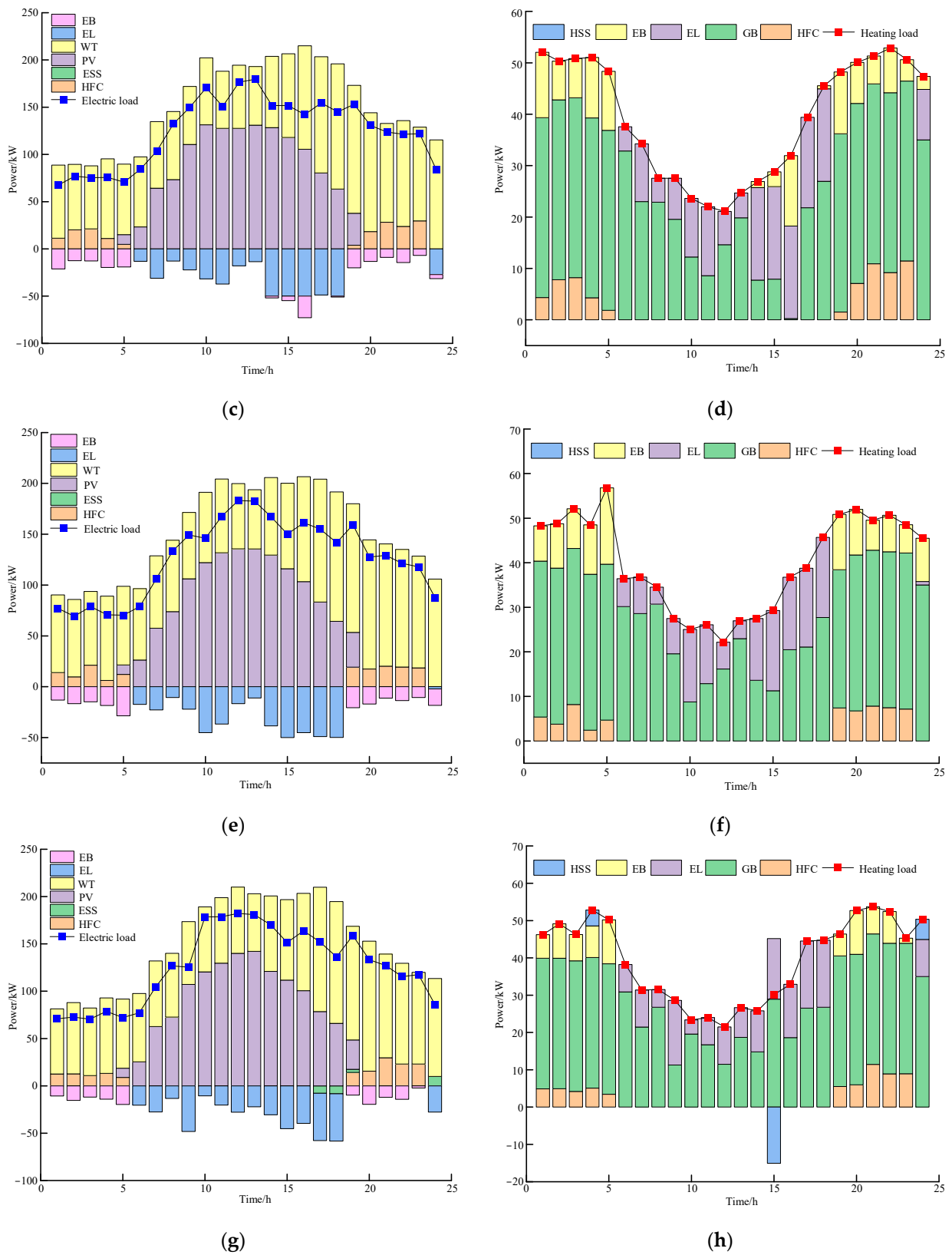
Figure 6. Results of electricity, heat balance scheduling: (a) Electrical Balance Diagram for Scene 1; (b) Heat Balance Diagram for Scene 1; (c) Electrical Balance Diagram for Scene 2; (d) Heat Balance Diagram for Scene 2; (e) Electrical Balance Diagram for Scene 3; (f) Heat Balance Diagram for Scene 3; (g) Electrical Balance Diagram for Scene 4; (h) Heat Balance Diagram for Scene 4.
