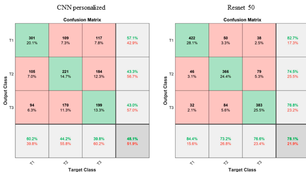
Figure 3. Confusion matrix between neural network-based models for classification of nitrogen doses in strawberry floral induction. In green (main diagonal) are the true positives of each class. In salmon, horizontally there are false negatives, and vertically the false positives. In light and dark gray are accuracies and errors by classes and total respectively.
