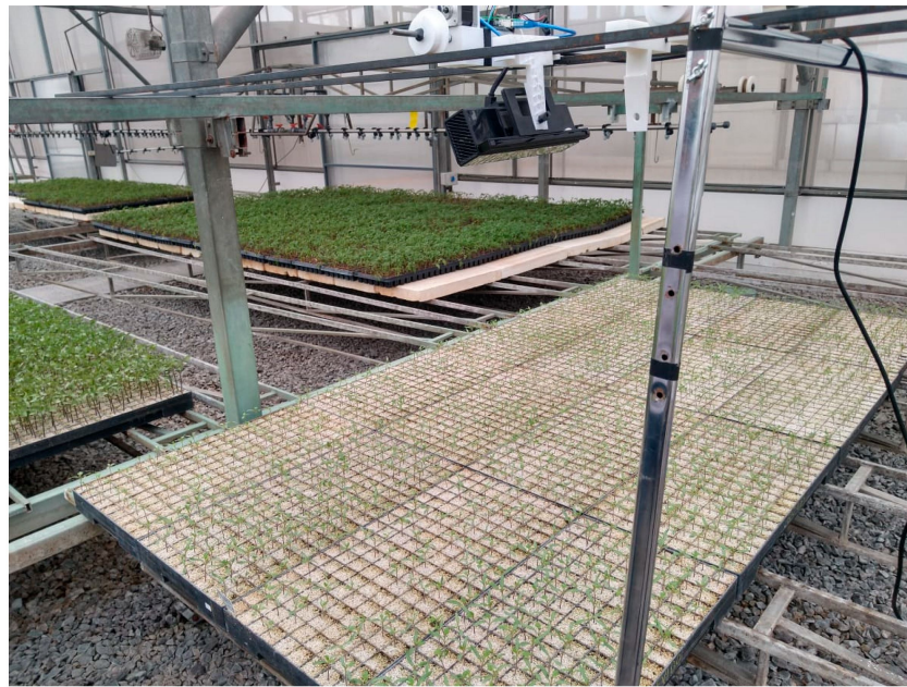
Figure 1. ScanSeedling v2.0: prototype scan of entire crops. The sensor moves along the x -axis to 2 m, the y -axis to 6 m, and the z -axis to a height of 0.60 m.
