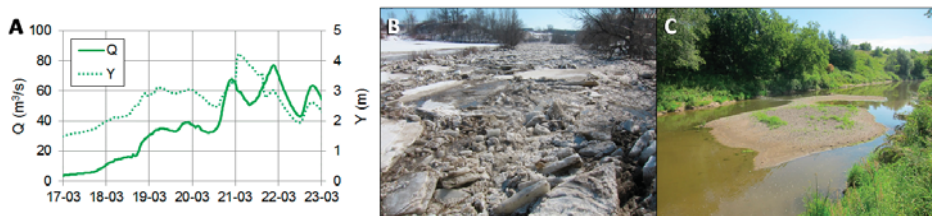
Figure 7. (A) Measured water depth ( Y ) and estimated discharge ( Q ) at breakup on the third order channel E3 showing the signature of an ice jam; (B) ice jam (photograph taken on 21 March 2012) and (C) new gravel bar formed where the jam toe had been momentarily located (photograph taken on 1 August 2012).
