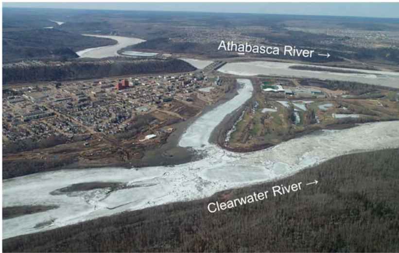
Figure 4. An aerial photo taken 8 April 2015 showing the confluence of the Athabasca and Clearwater rivers in close proximity to downtown Fort McMurray, when there was an ice jam several kilometres along the Athabasca River and an intact ice cover on the Clearwater River (courtesy of Gov't of Alberta).
