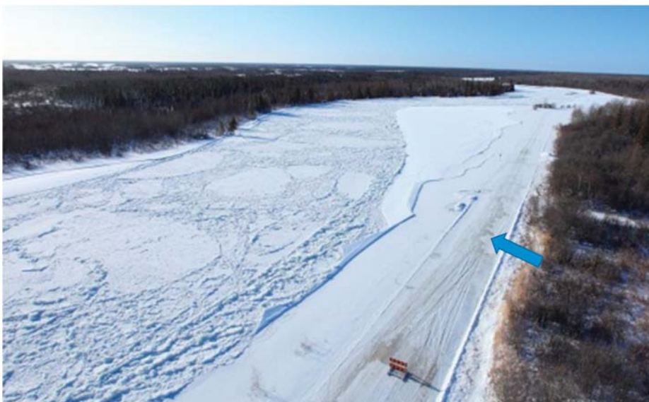
Figure 6. Encroached floodwater frozen to road surface, as indicated by the arrow. The road surface profile was surveyed before the flood event so that the backwater elevation could be determined at the time of the flight.
