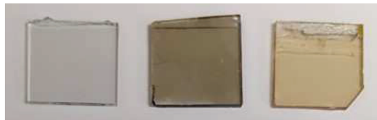
Figure 7. Appearance (from left to right) of: initial FTO-coated glass substrate, as-deposited 60 nm thin films, annealed 60 nm thin film (note that the silver area at the top is silver paint and not part of the sample).
