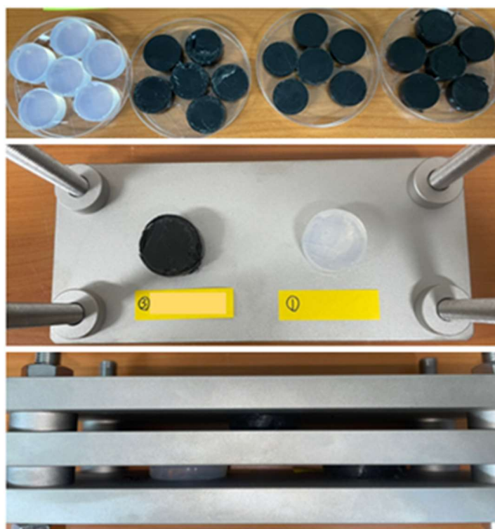
Figure 3. Compression set test jig and specimens.
