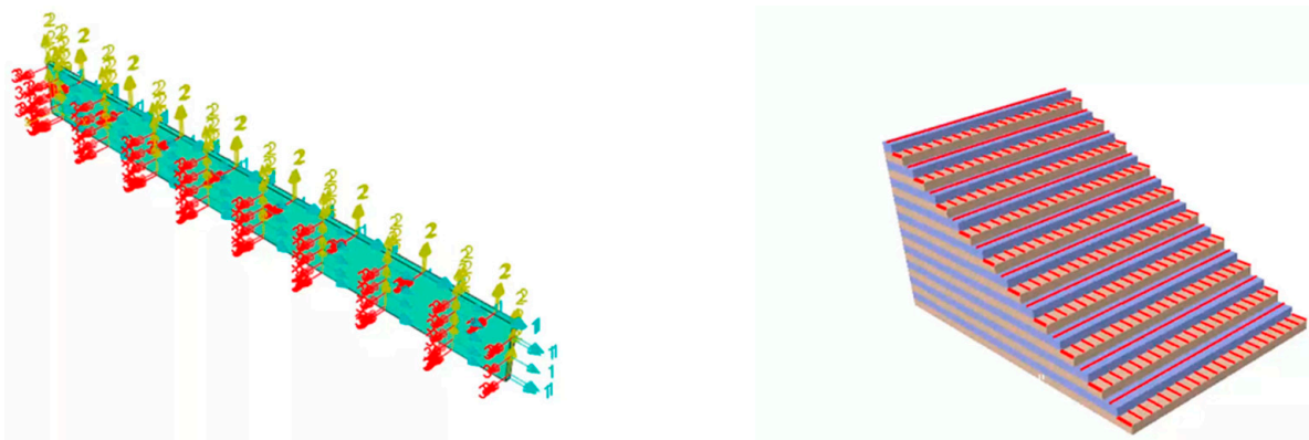
Figure 1. Lamination sequence of CFRP laminated plate.
