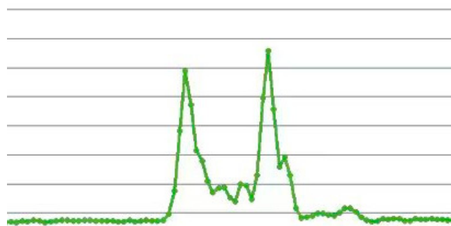
Figure 20. Chirping phenomenon of the FBG waveform.
