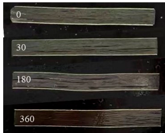
Figure 8. Interlayer cracks before and after hygrothermal accelerated aging.
