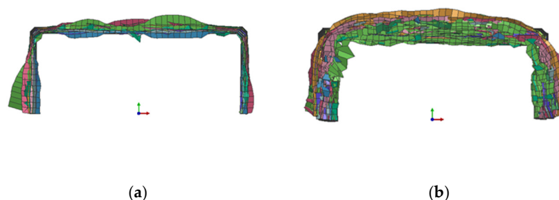
Figure 16. Delamination (a) and folding deformation (b).
