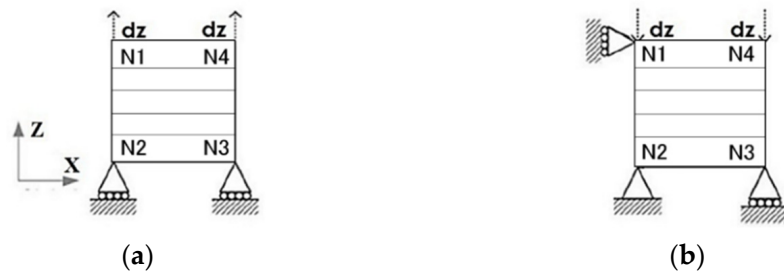
Figure 6. Tension load (a) and compression load (b).
