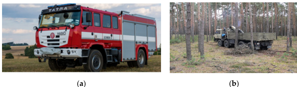
Figure 5. Fire and tested vehicles. (a) Fire vehicle Tatra 815 4 × 4, Length/Width/Height: 7950/2550/3000 mm. (b) Tested terrain vehicle Tatra 815 8 × 8, Length/Width/Height: 8950/2550/3300 mm.
