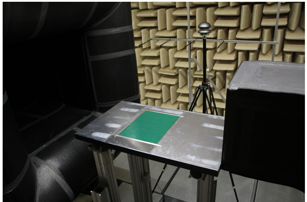
Figure 7. Photo of the measurement setup for the first tests under flow conditions. The MEMS array is mounted on the plate that is used as an extension of the bottom wind tunnel wall.
