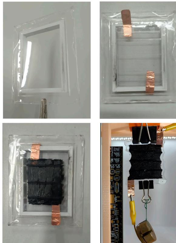
**Figure 6.** The step-by-step fabrication process of the DEA.
