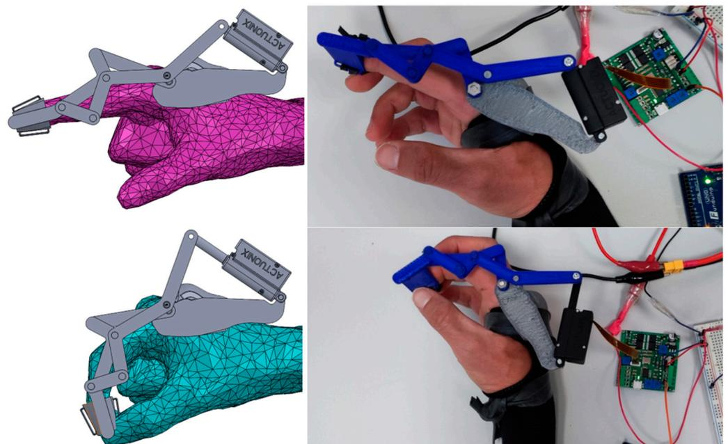
Figure 13. Final design and testing of the RHEx.
