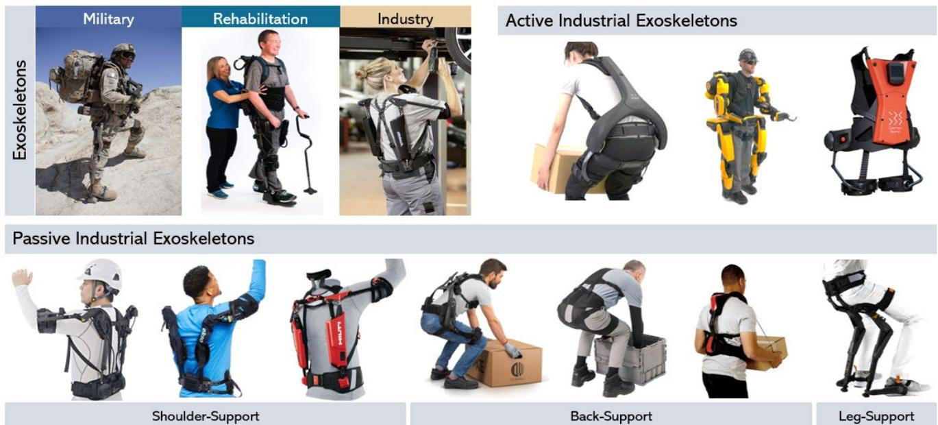
**Figure 1.** Application areas of exoskeletons (top-left), active (top-right) and passive (bottom) industrial exoskeletons classified into the shoulder, back, and leg support exoskeletons (adapted from [9]).
