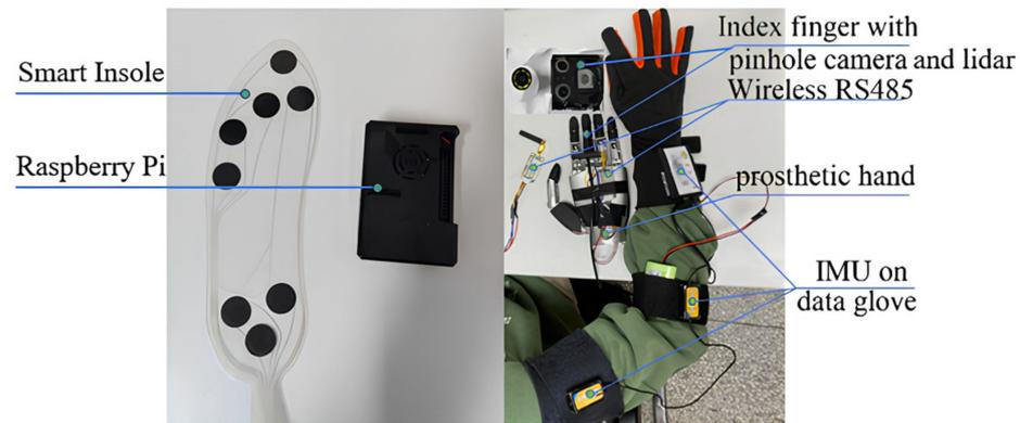
Figure 1. Hardware composition of the prosthetic hand control system.
