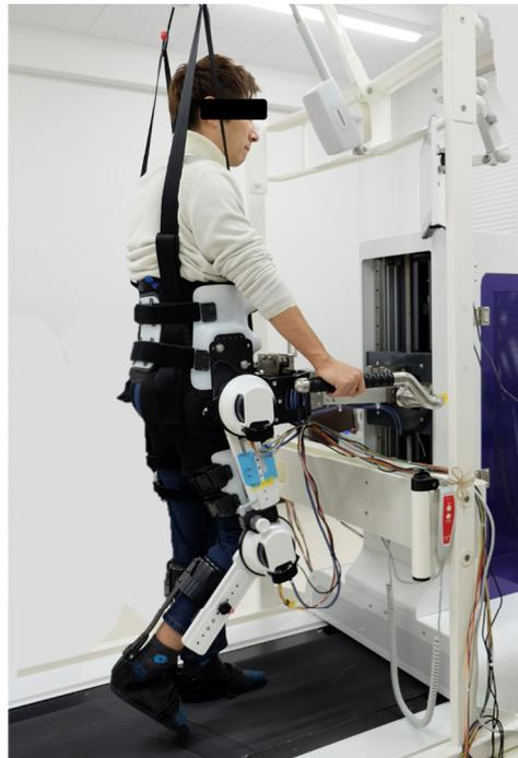
**Figure 1.** Gait exercise rehabilitation robot. The robot has an exoskeleton, rehabilitation lift, treadmill, and functional electrical stimulation (FES).
