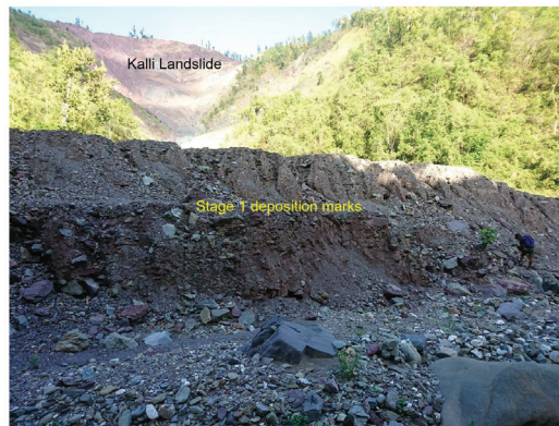
Figure 6. The deposition marks remained at the sides after the debris from the first stage. The location is 600 m from the landslide crown.
