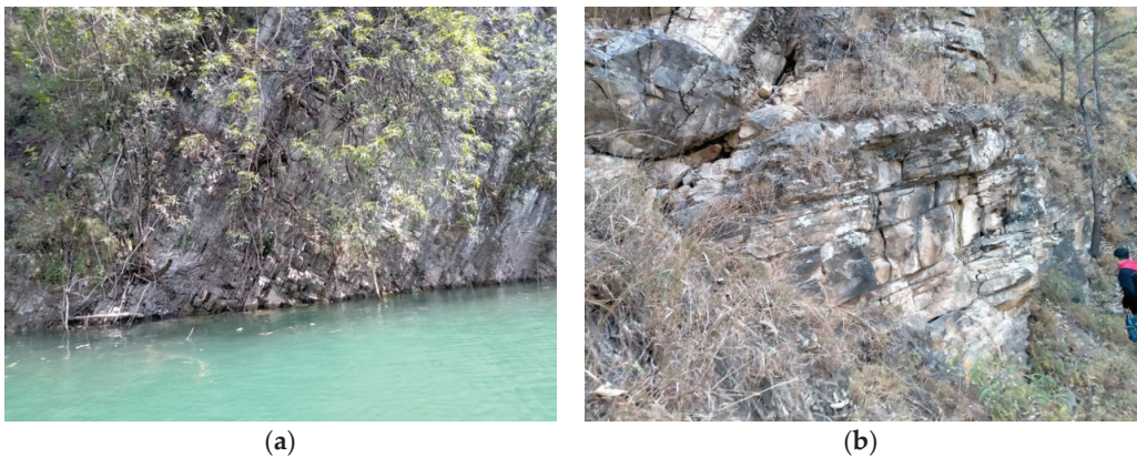
Figure 7. Toppling rock mass of the bank slope. (a) Near the reservoir surface at 1403 m; (b) at the elevation of 1540 m.
