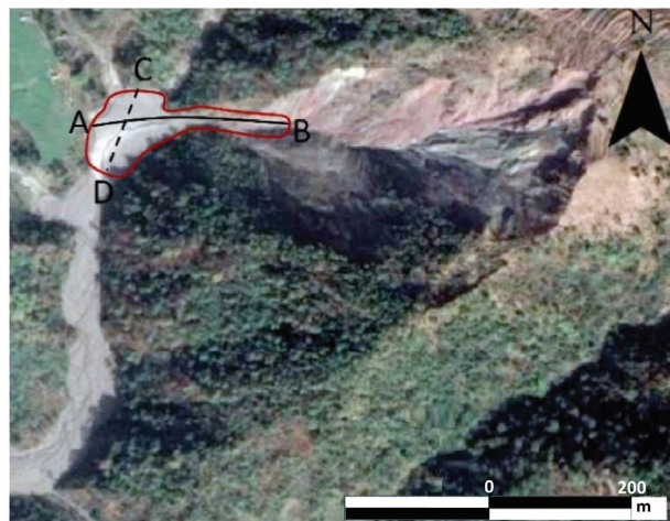
Figure 9. Deposition area (marked in red) of debris material near Pipaltada village (Figure 5), accumulated during the first stage, as observed in the field. Deposition along the longitudinal direction, AB, and the transversal direction, CD, is examined in the subsequent simulation.
