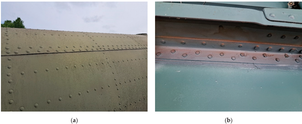
Figure 4. Examples of riveted lap joints in the tested helicopter: views from the outer (a) and inner (b) sides.
