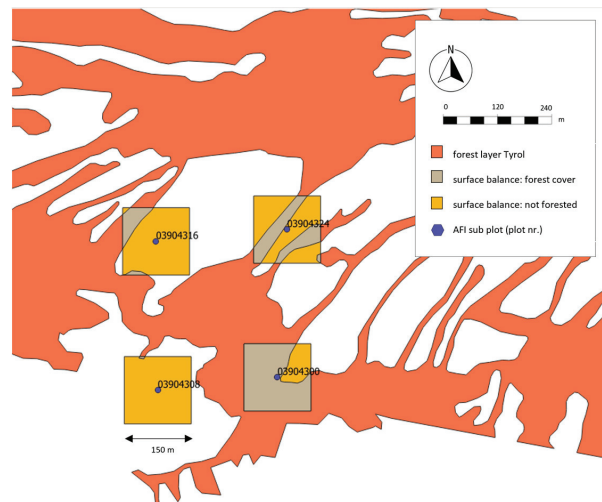
Figure 5. Assessment of surface balance (47°15′34.7724″ N, 11°24′1.3500″ E). Squares with side length 150 m are used to compute surface balance around AFI subplots (e.g., plot nr. 03904308) between forest (light orange polygons) and non-forest area (grey polygons) in QGIS.
