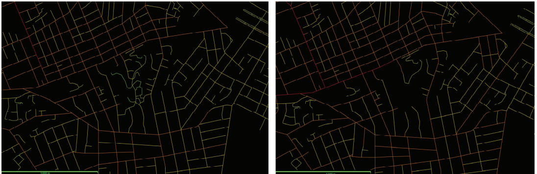
Figure 11. The area of the current Shadyside Campus at the beginning of the 20th century (simulation)—integration map (left). Shadyside Campus, PA, nowadays—integration map (right). The degree of integration for each segment line is depicted using a color scale. The red axes denote the highest integration; green signifies the lowest. The levels between the highest and lowest are gradually shifting. Space Syntax analyses by Z. Bereczki, 2023.
