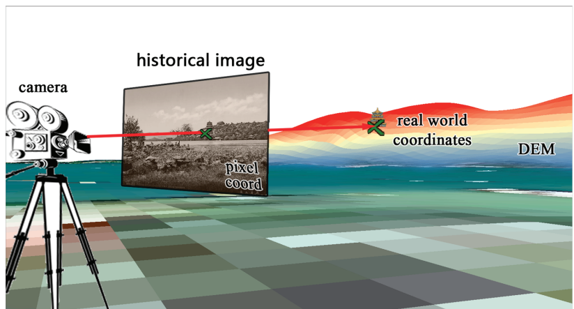
Figure 4. Schematic diagram of the WSL Monoplotting Tool.
