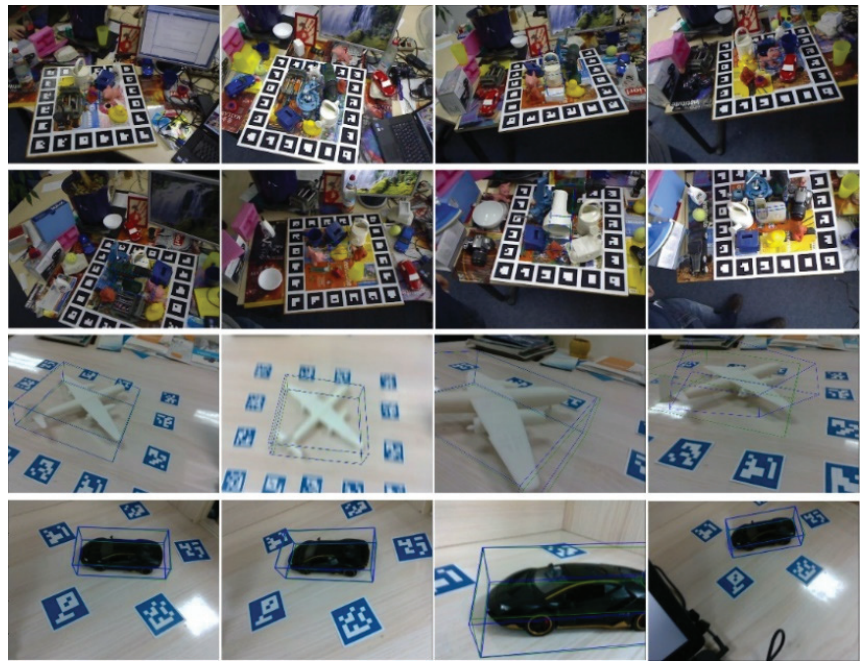
Figure 10. Visualization results of pose estimation using our method on the dataset. The green box outlines indicate the ground truth object pose information while the blue box outlines indicate the estimated object pose information obtained through inference. The top two rows display the pose estimation results of some objects in the LineMOD dataset while the bottom two rows demonstrate the performance on the airplane and car model datasets, including the handling of blur, illumination variations, viewpoint changes, scale variations, and occlusion, as well as instances of erroneous estimations.
