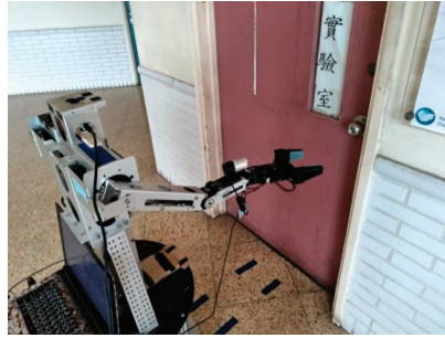
Figure 16. The robot arm lifts to the specified height; the Chinese characters on the figure are the room's name.
