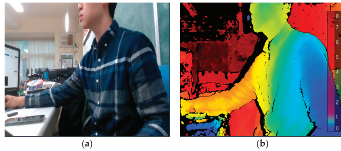
Figure 7. (a) is the original image, (b) is the depth image where the blue color means the object is near to the camera, and dark red means the object is far from the camera. The distance ranges from 0 m (dark blue) to 8 m (dark red).
