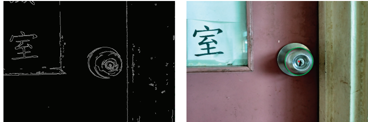
Figure 10. Edge detection uses a threshold, and the doorknob is detected; the Chinese character on the left part of the figure is the room's name.
