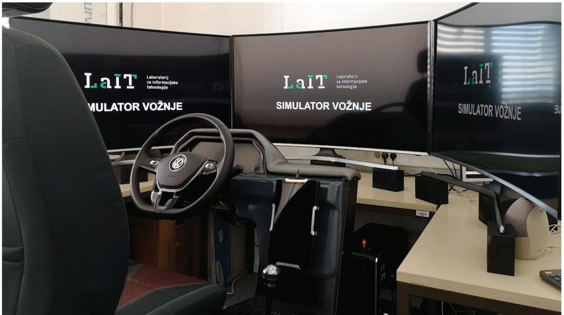
Figure 1. NERVtech™ motion-based driving simulator located at the University of Ljubljana, Faculty of Electrical Engineering.
