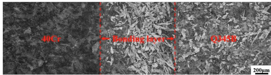
Figure 10. Interfacial microstructure of 40Cr/Q345B bimetallic ring blank [77].
