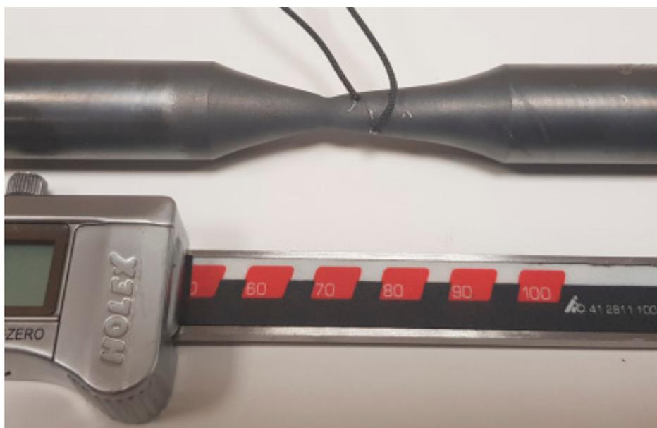
**Figure 18.** The view of the 20MnB4 steel sample after the deformation process in a complex deformation state (simultaneous torsion and tension) and location of the deformation outside the test area.
