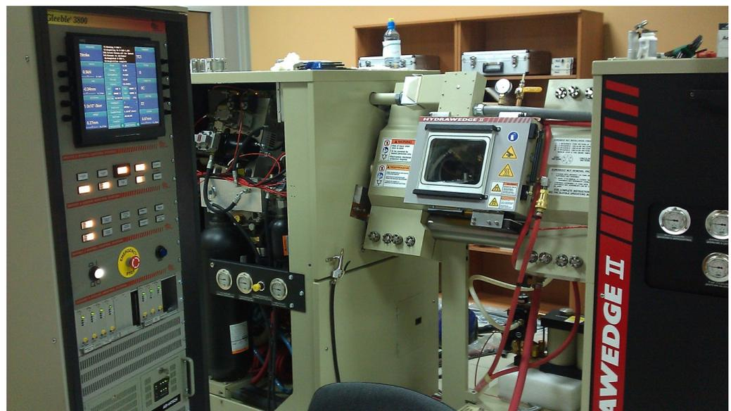
Figure 2. The Gleeble 3800 plastometer testing equipment.
