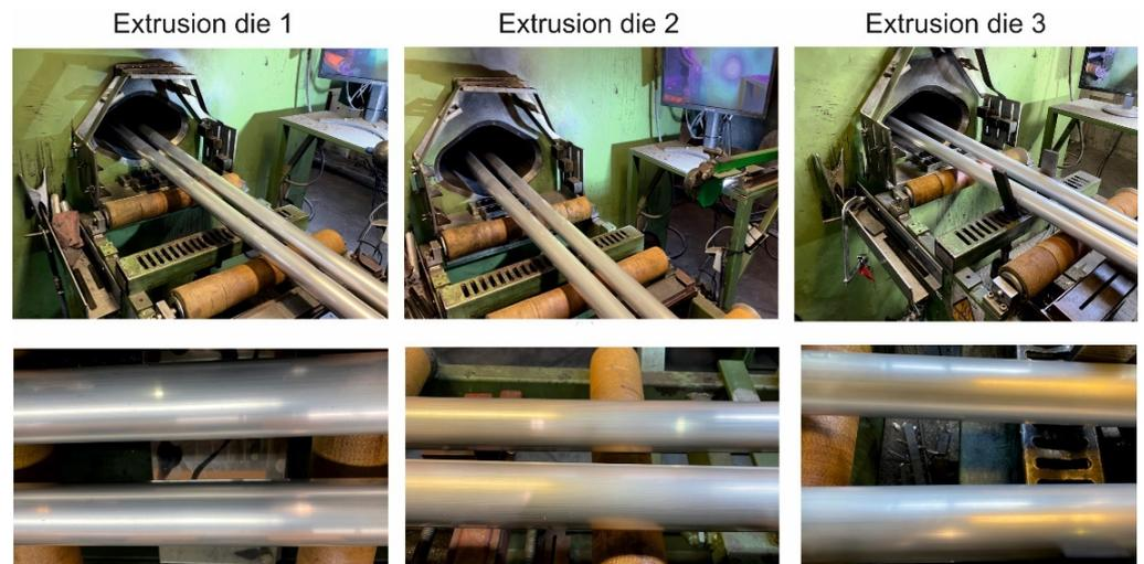
**Figure 12.** Extruded tubes of  $\text{Ø}50 \times 2$  mm from 7021 alloy on the press run-out table for dies of different geometry: die 1,  $T_0 = 480$  °C,  $V_1 = 4.5$  m/min; die 2,  $T_0 = 480$  °C,  $V_1 = 3.5$  m/min; die 3,  $T_0 = 480$  °C,  $V_1 = 4.5$  m/min.
