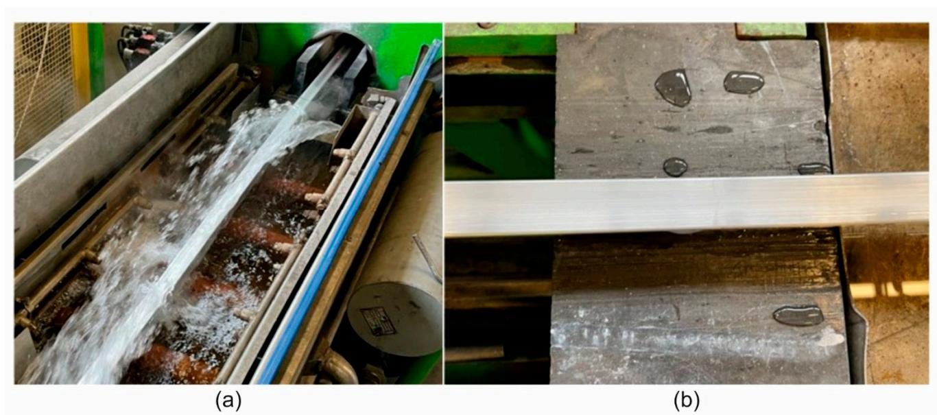
**Figure 5.** The 5 MN 4-inch extrusion press run-out table with water wave installation (a) and the profile from AlMgSi(Cu) alloy after extrusion with cooling by water on the run-out table (b).
