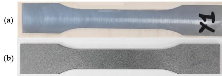
**Figure 14.** Example of a test sample: (a) before painting, (b) after painting.
