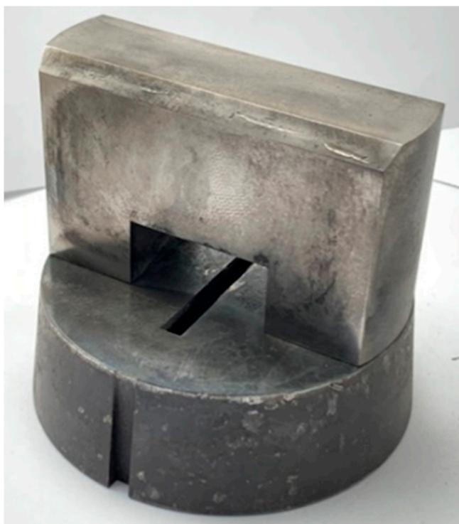
**Figure 2.** A die insert with single bridge used for extrusion of 60 × 6 mm flat bar with weld.
