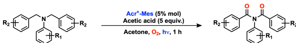
Scheme 19. \text{Acr}^+ -Mes-photocatalyzed aerobic photooxygenation of N,N -dibenzylanilines to imides.
