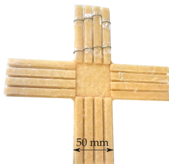
Figure 7. Image of the cruciform specimen with bonded reinforcements on the arms, thickness of the area of interest: 2 mm.
