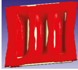
Figure 12. The draped part shown as charge layover the cavity.
