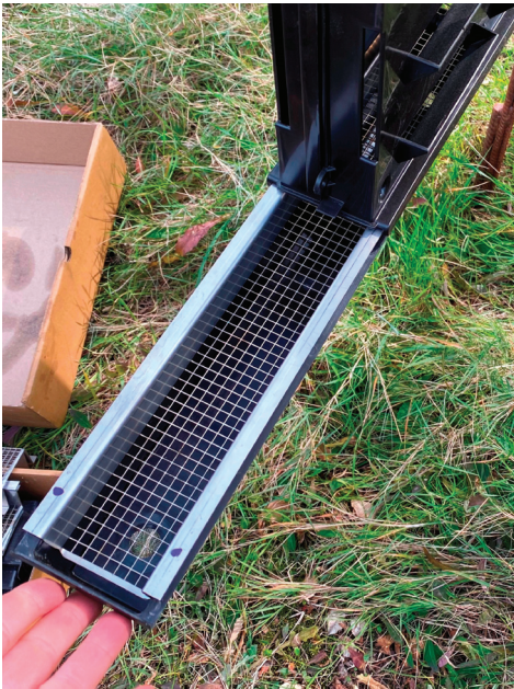
Figure 2. Modification with a steel mesh with a 6 mm screen.
