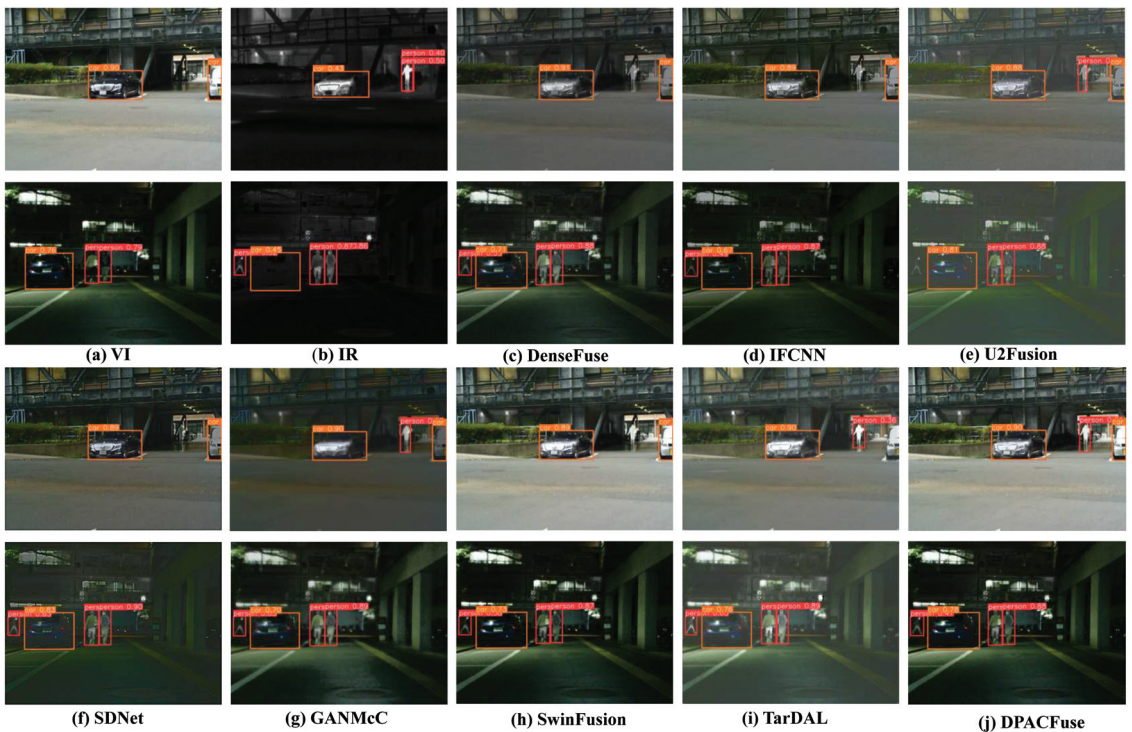
Figure 10. Object detection results on the MSRS dataset. The results are provided for two scenes from 00479D (top) and 01348N (bottom), respectively.
