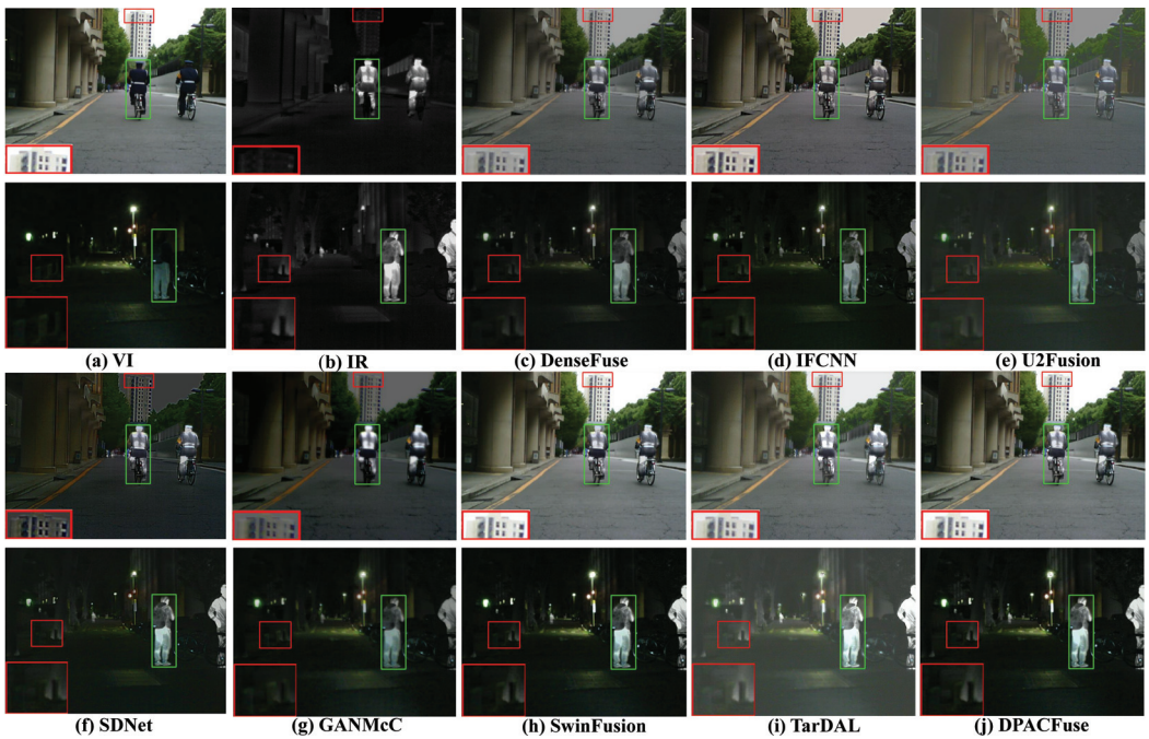
Figure 3. Qualitative analysis of DPACFuse with seven methods on 00537D (top) and 01012N (bottom) images from the MSRS dataset.
