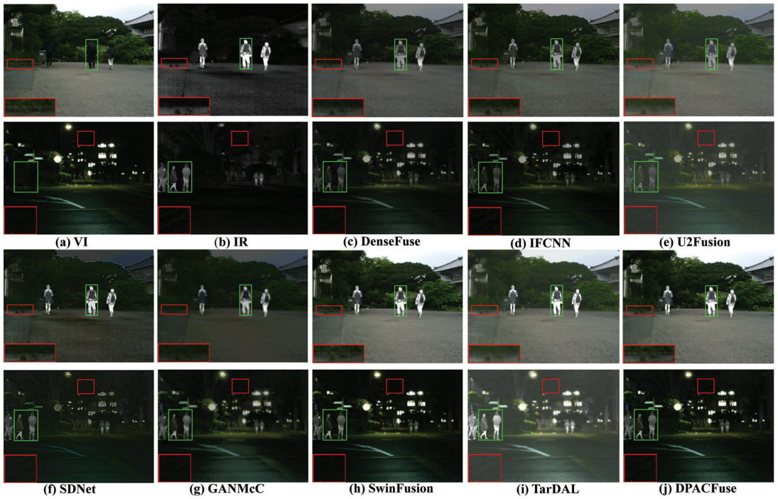
Figure 2. Qualitative analysis of DPACFuse with seven methods on 00634N (top) and 01356N (bottom) images from the MSRS dataset.
