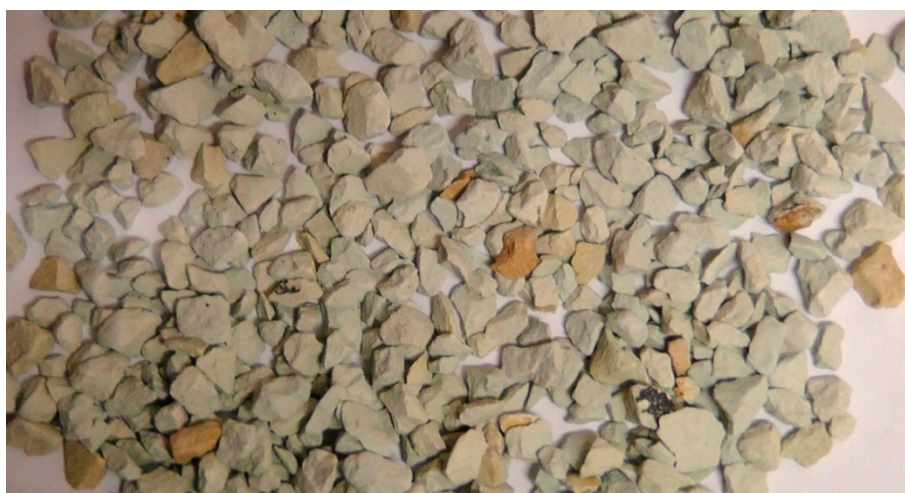
Figure 1. Zeolite clinoptilolite with a grain size from 2.5 to 5 mm.
