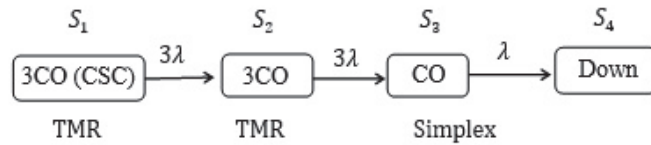
Figure 7. Markov chain for TMR/Simplex and one CSC ( k = 4 ).
