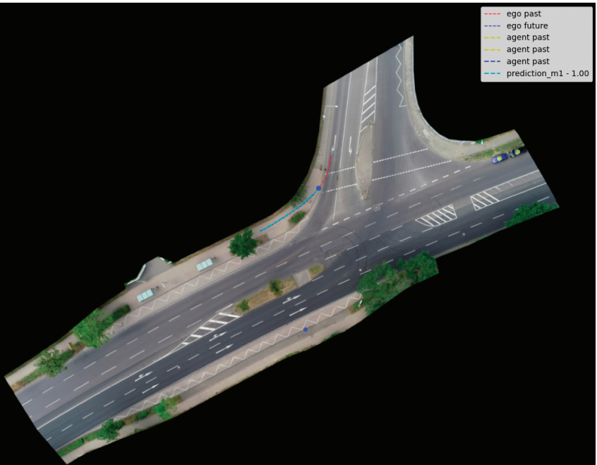
Figure 14. Traffic scene prediction with the unimodal approach. In this scenario, the bicyclist is going to the sidewalk part of the road.
