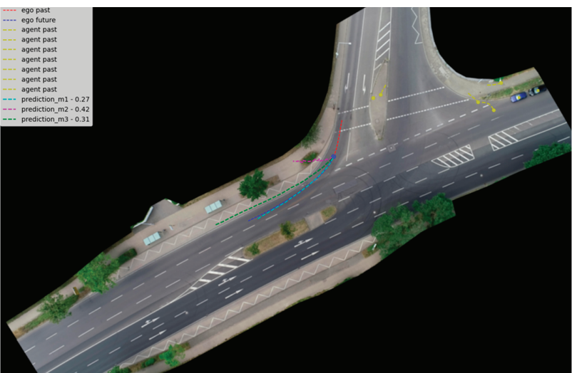
Figure 17. Traffic scene prediction with the multimodal approach. In this scenario, the bicyclist has the most probable maneuver drawn with magenta (going to the sidewalk), the second one drawn with green (going to the bus station), and the third one drawn with blue (following the lane).
