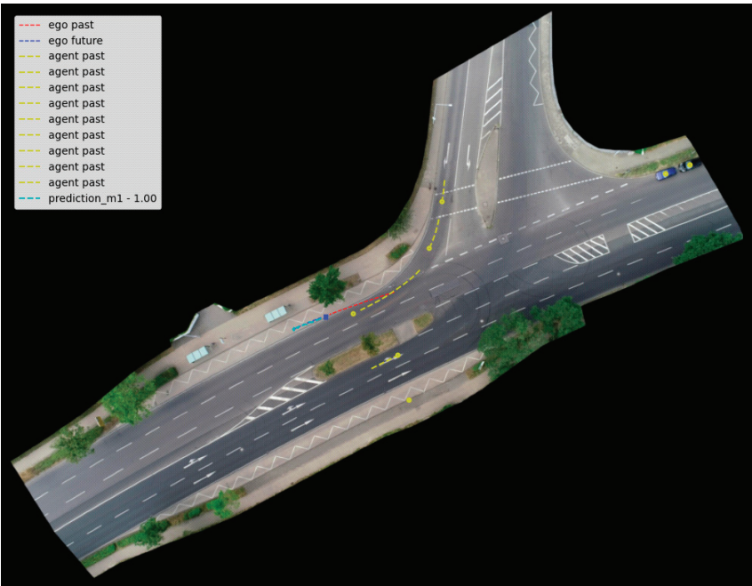
Figure 13. Traffic scene prediction with the unimodal approach. In this scenario, the bus is stopping at the bus station.
