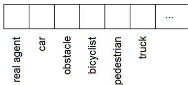
Figure 3. The identification of an agent. Each of the six attributes of the input instance has a binary value designating the presence or absence of a feature. The first attribute is 1 if the block identifies a real agent and 0 if it identifies a dummy agent. The following five attributes constitute a one-hot encoding of the agent type, e.g., the second attribute is 1 if the agent is a car and 0 if it not a car, and so on.
