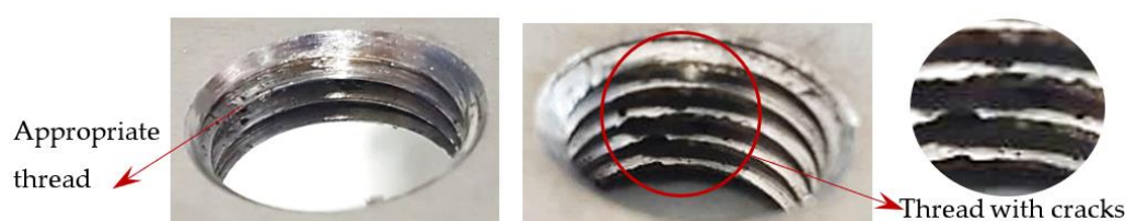
Figure 2. Internal thread M10 on the left without cracks in 5 mm thick sheet metal, and, on the right, with cracks in 10 mm thick sheet metal.
