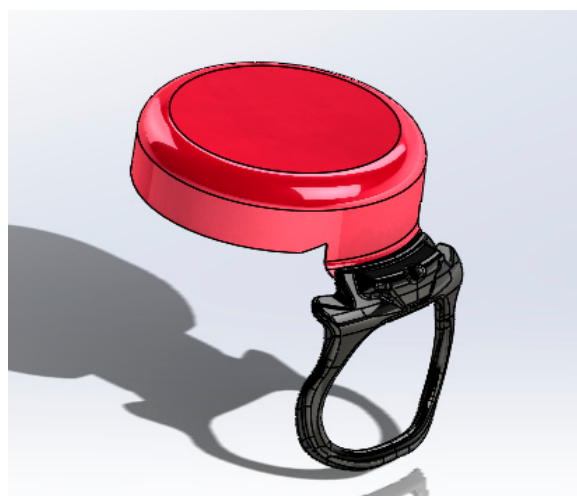
Figure 1. Exemplary geometry of lacquered pull-off cap.
