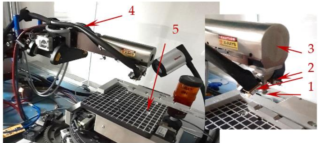
Figure 6. Device for measuring residual stresses Proto iXRD (laboratory setup): 1—collimator directing the X-ray beam; 2—a pair of detectors capturing the diffraction cone; 3—X-ray tube with Cr target; 4—Cobralink ® flexible measuring arm; 5—adjustable and rotating table.
