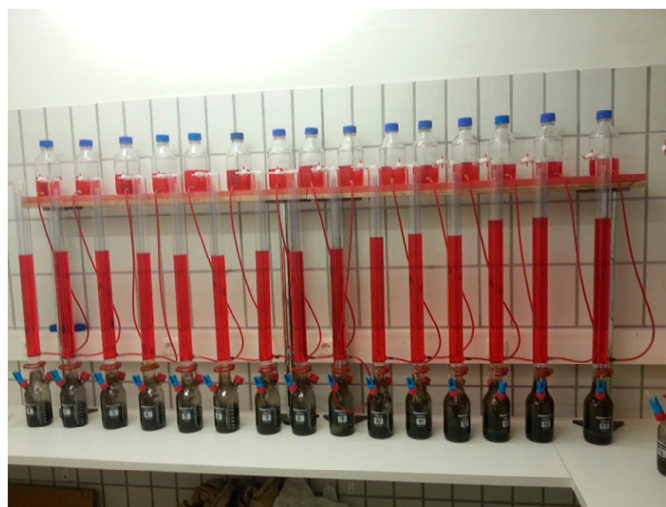
Figure 1. Laboratory setup for evaluation of the RGP in specific sludge samples using eudiometric tubes.
