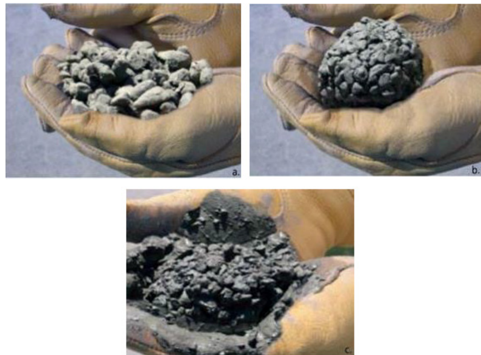
Figure 5. Hand compacting method: (a) scarce water content; (b) adequate water content; (c) excess water content (copyrighted from [124]).
