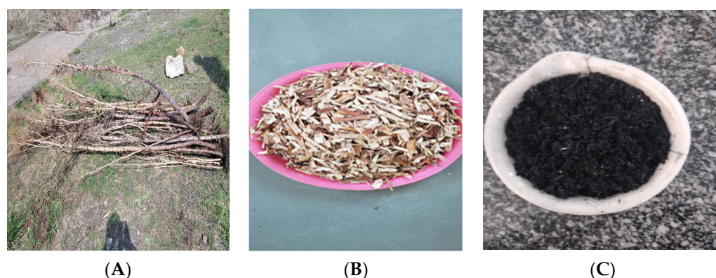
Figure 2. RAB preparation stages: (A) stem of Rumex abyssinicus , (B) partially size-reduced sample and (C) ready-made adsorbent.
