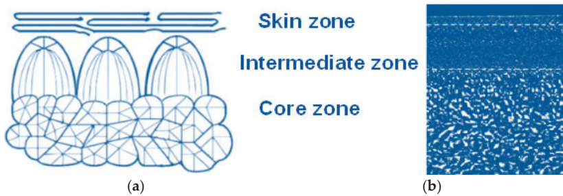
Figure 1. Morphological structure: (a) scheme of skin–core structure; (b) optical microscope—skin–core structure.
