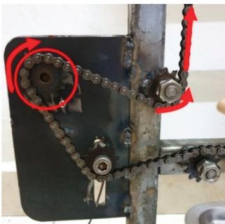
(c) Sprocket configuration on the motor bracket
