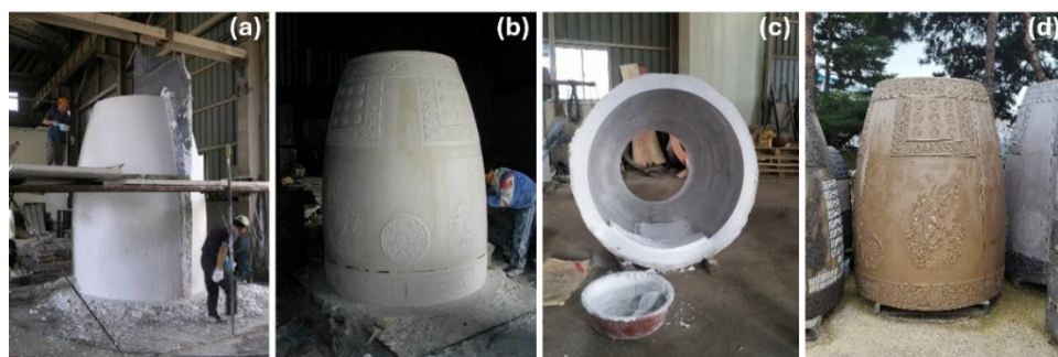
Figure 13. The fabrication process of a bell form. (a) A POP bell form, (b) an engraved plaster bell form, (c) an intaglio FRP bell form, and (d) a completed bell form.
