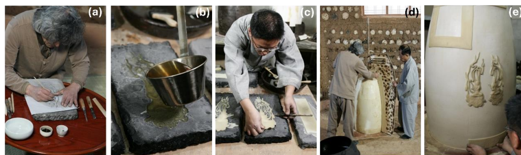
Figure 9. The fabrication process of a beeswax form [110,116]. (a) Pattern engraving, (b) beeswax pouring, (c) beeswax patterning, (d) plane beeswax form, and (e) beeswax bell form.
