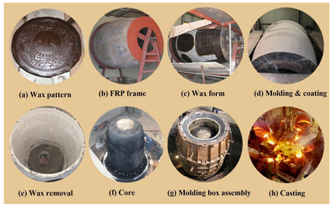
Figure 10. The LWC method used to produce a temple bell. (a) Wax pattern, (b) FRP frame, (c) wax form, (d) molding and coating, (e) wax removal, (f) core, (g) molding box assembly, and (h) casting [122].
