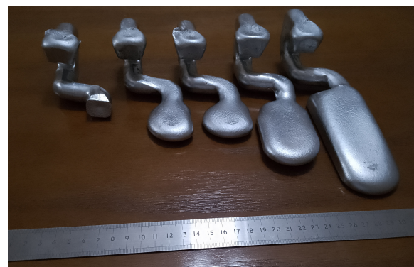
Figure 5. Runner and samples of rheocast A356 from left to right at 615 °C, 630 °C, 660 °C and 690 °C, respectively, made using horizontal SCP.
