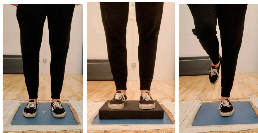
Figure 1. (Left): A participant standing on the force platform on both feet during the clinical test of sensory interaction and balance (CTSIB) test; (Middle): A participant standing on a foam pad placed on the force platform on both feet during CTSIB test; (Right): A participant standing on the force platform on one foot during unilateral stability test.
