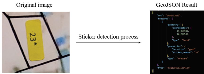
Figure 4. An example of the output from the sticker detection process.
