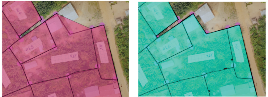
Figure 3. Examples of the convex hull method and the GRASS method, respectively.
