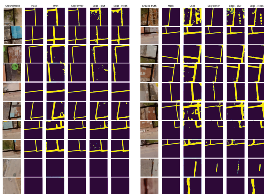
Figure 6. Examples of boundary predictions on the test dataset. Patches where the whole boundary is correctly predicted ( left ); patches where the boundary is not correctly predicted for at least one of the techniques ( right ). The boundaries predicted at the patch level are then merged (and post-processed to close gaps) to obtain the parcels for a whole study area.
