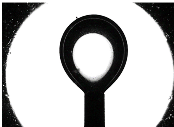
Figure 3. IFT measurement using Pendant drop method.
