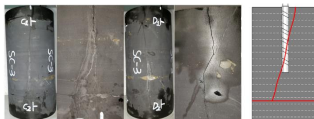
Figure 26. Core photos and acoustic emission location results of sample 9 after the experiment.
