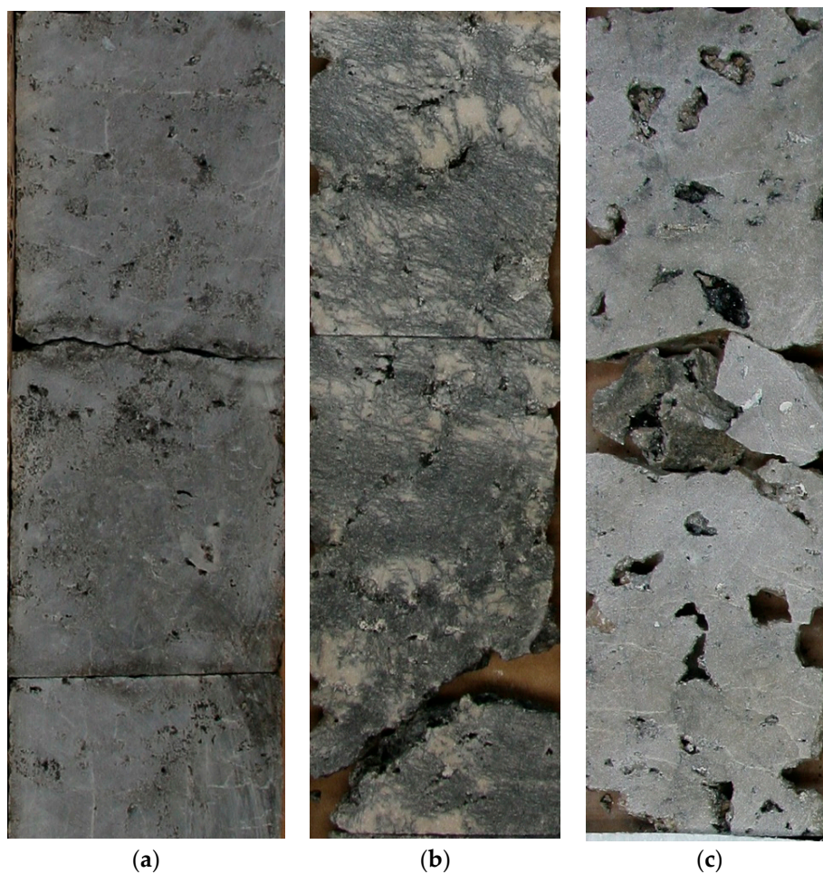
Figure 6. Vuggy pores in Famennian reef reservoirs: (a)—small vuggy pores; (b)—medium-sized vuggy pores; (c)—large vuggy pores.
