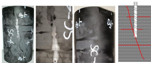
Figure 28. Core photos and acoustic emission location results of sample 10 after the experiment.
