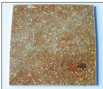
Figure 1. Chicken feather/PLA biocomposite containing 50 wt % of feather.
