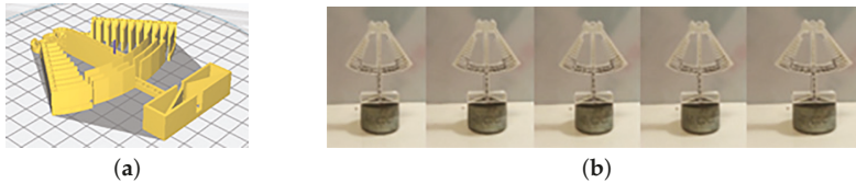
Figure 8. Magnetic actuation at the macroscale: (a) bulk stl file (left and right wings); and (b) motion sequence of the armed wings.
