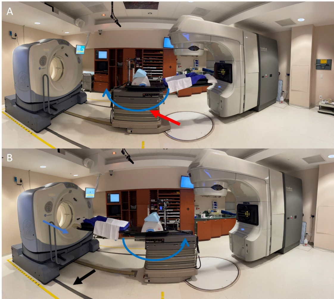
Figure 3. Photos of the CTOR–linac set up. First the patient is set up in the treatment position, with the couch positioned in the linac position (A) and BBs are placed in the laser positions. The base of the couch (red arrow) is then rotated 180° (curved blue arrows), according to the CT scanner position (B). The CT scanner moves along the rails on the floor (black arrow) in the direction of the straight blue arrow to take a scan. After image alignment, the patient is rotated back to the linac position and the lasers are aligned with the BBs. Final couch shifts are made from this position.
