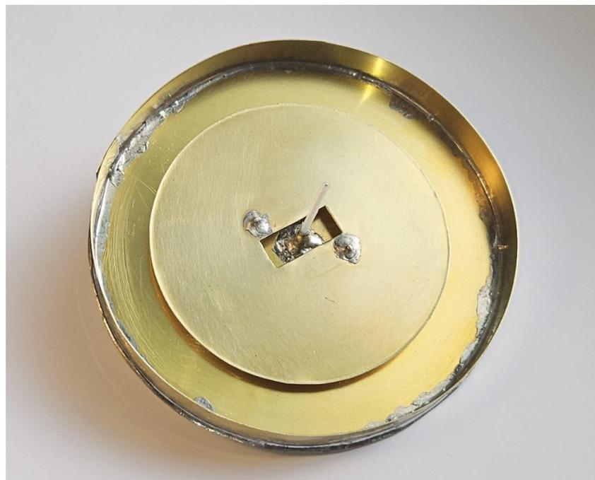
**Figure 3.** A fabricated prototype of a patch-monopole monopulse feed.
