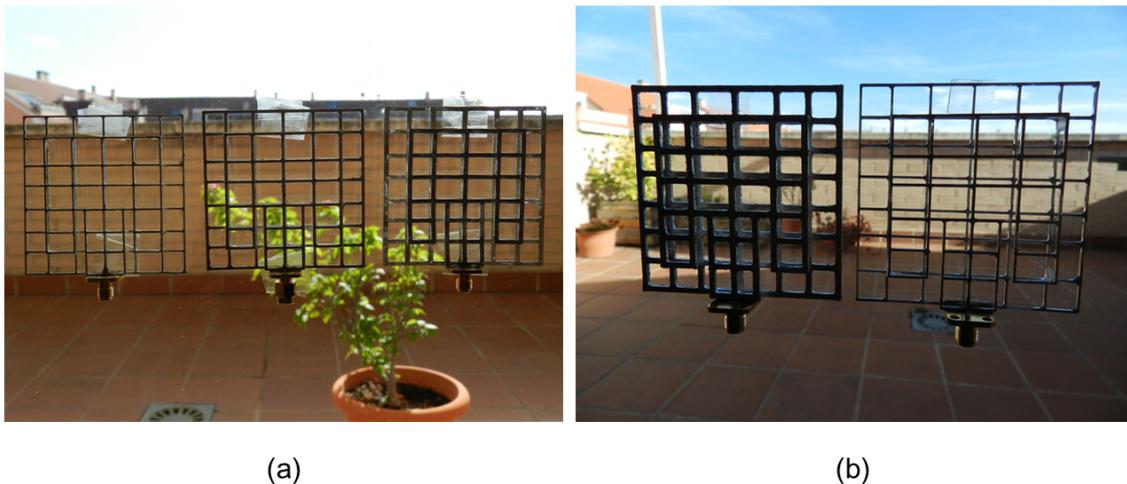
**Figure 22.** Photographs of prototypes placed on a window to showcase their transparency, manufactured with: (a) PET and widths of  $d = 0.5$  mm (left) and  $d = 1$  mm (center); with resin and a width of  $d = 2$  mm (right); (b) PLA and a width of  $d = 2$  mm (left); and PET and a width of  $d = 0.5$  mm (right).
