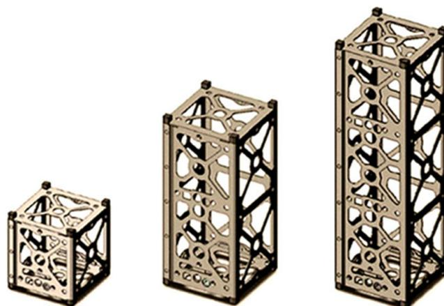
**Figure 2.** CubeSat designs: (left) 1U; (middle) 2U; (right) 3U [1].
