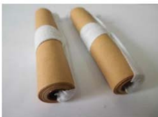
Figure 3. The capacitor core model of condenser bushing.
