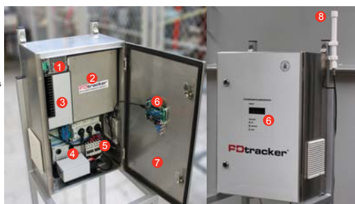
Figure 1. Hardware architecture of a prototype online partial discharge (PD) monitoring system for power transformers.
