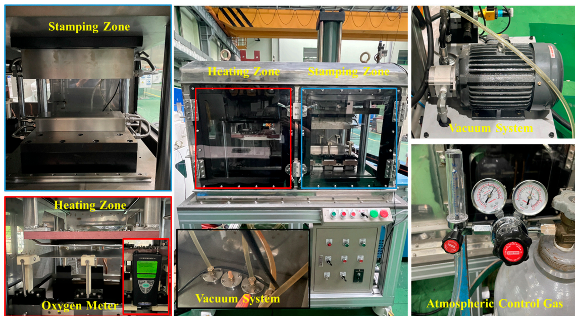
Figure 12. Lab-scale hot stamping simulator.
