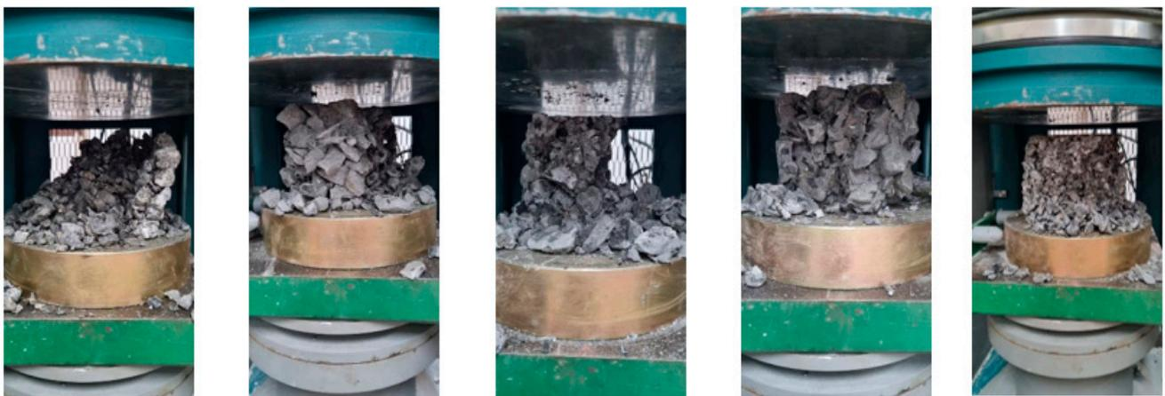
Figure 5. Ultimate failure modes of cube specimens.
