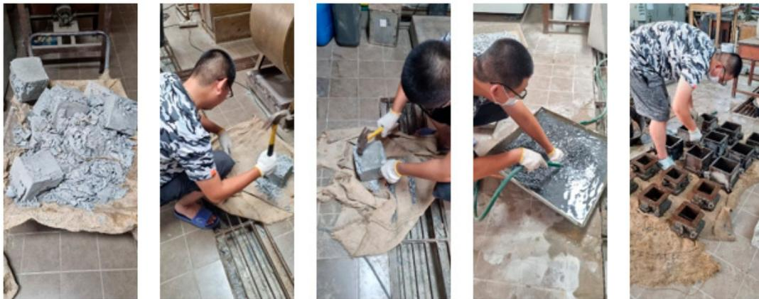
**Figure 1.** Acquisition of recycled aggregates in process.
