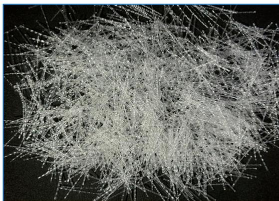
Figure 1. Polypropylene fibers used.
