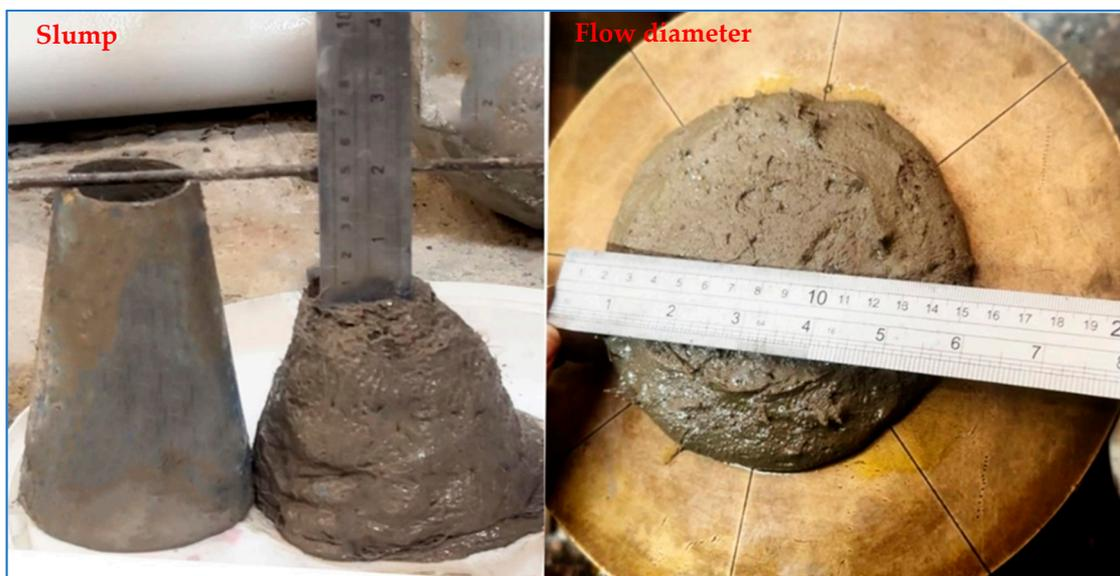
**Figure 4.** Measuring of EGC workability.
