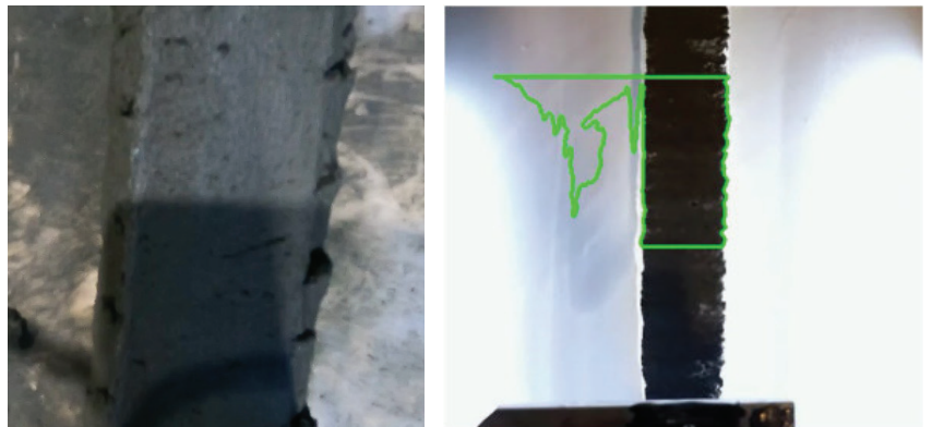
Figure 10. Left: Image sample by SC3DP taken by a camera attached to the nozzle, displaying background noise (splatters and residuals of concrete). Right: Error in feature extraction where background features were highlighted with a green outline (inclusive of the concrete filament), resulting in a discarded image (Image from Kazemian et al. [18]).
