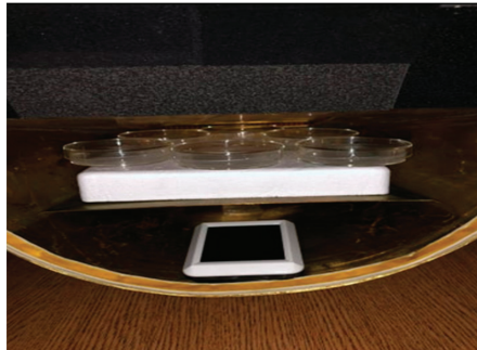
Figure 1. Gigahertz transverse electromagnetic (GTEM) chamber. View of the GTEM chamber in which the boar semen samples were placed together with a digital thermometer.
