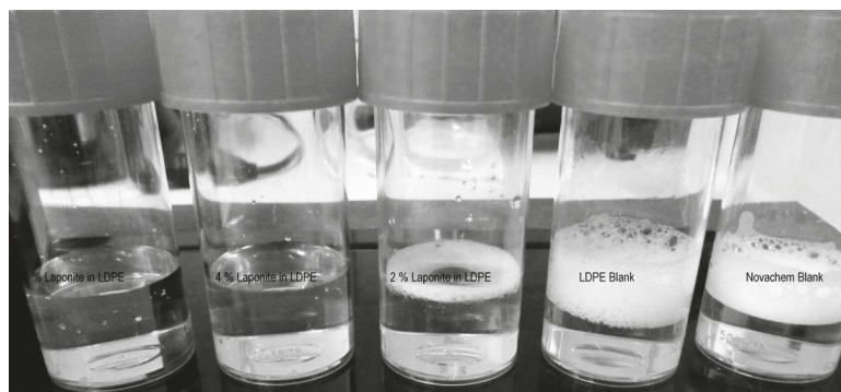
Figure 6. Migration samples after they were shaken. From left to right: 6% Laponite in LDPE, 4% Laponite in LDPE, 2% Laponite in LDPE, LDPE blank and the surfactant blank used as food simulant for all migration samples.
