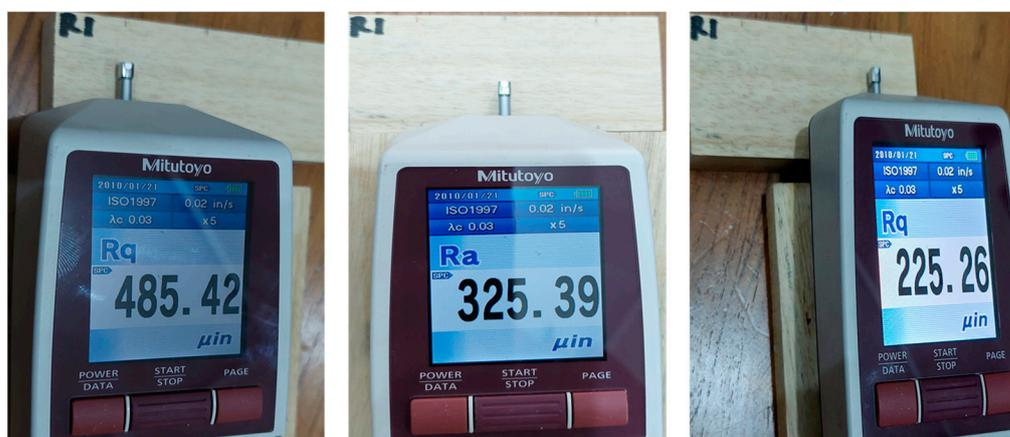
**Figure 1.** The surface roughness measurement of Jabon wood specimens in three different positions using a portable stylus-type profilometer (Mitutoyo SurfTest<sup>®</sup> SJ-210).
