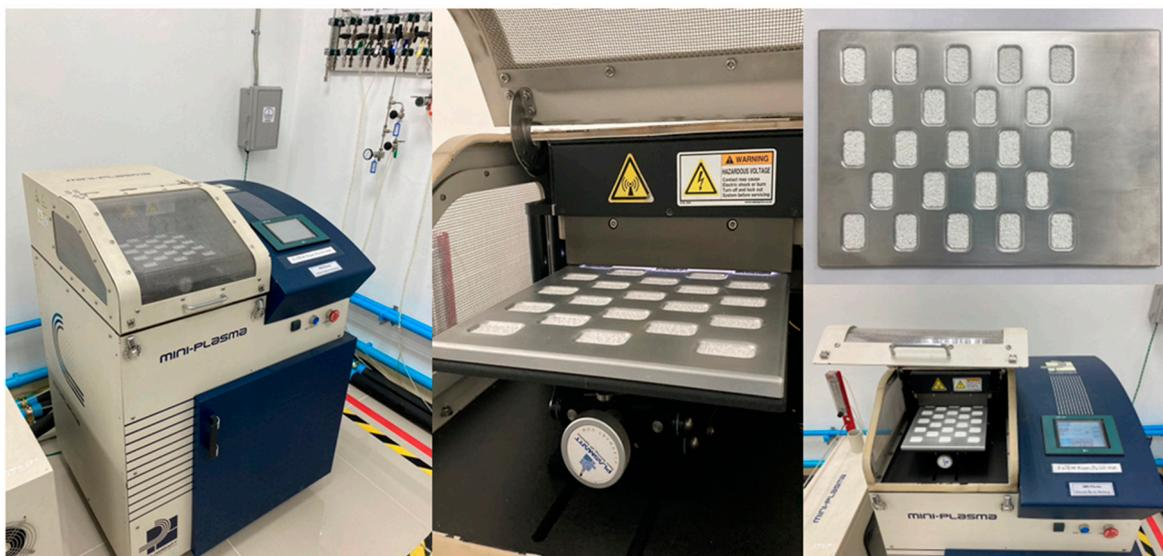
**Figure 1.** Dielectric barrier discharge (DBD) plasma machine.
