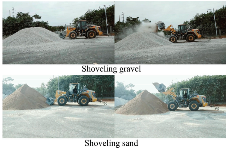
Figure 6. Shoveling gravel and shoveling sand.
