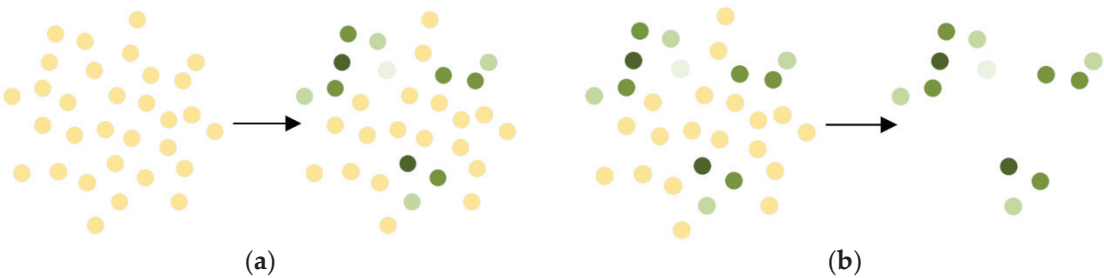
Figure 7. Particle weights and updating iterative particles, the weight of yellow particles is smaller than that of light green particles, and the weight of dark green particles is the largest: (a) update particle weights; (b) filter less weighted particles.
