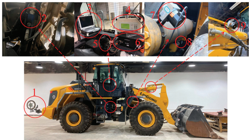
Figure 3. Automatic shoveling platform and sensors. As shown above, 1 fifth wheel gauge, 2 flow sensor, 3 vehicle PC system, 4 fifth wheel gauge control module, 5 signal receiving system, 6 all data acquisition system, 7 lift cylinder displacement sensor, 8 shoveling weight acquisition system, 9 tilt cylinder displacement sensor.
