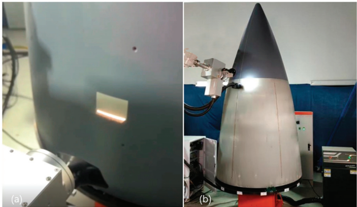
Figure 15. Laser cleaning: (a) the cleaning of a slice of workpieces and (b) the movement of the laser cleaning head between different slice layers.
