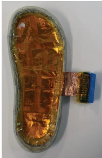
**Figure 6.** Assembled sensor installed on the outsole.
