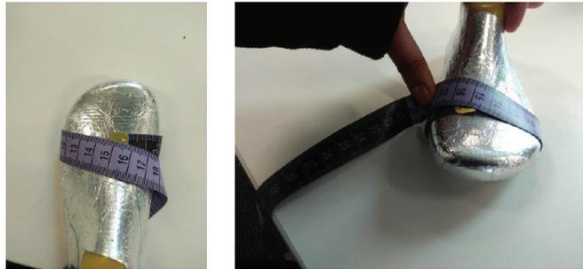
**Figure 21.** Tape measure wrapped around the widest part of the foot.
