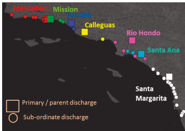
Figure 6. Locations and delineation of primary and sub-ordinate rivers and tributaries modeled in Southern California CoSMoS. Area-normalized runoff rates of primary (squares) discharge points were used to estimate discharge rates at sub-ordinate (circles of corresponding color) point locations.
