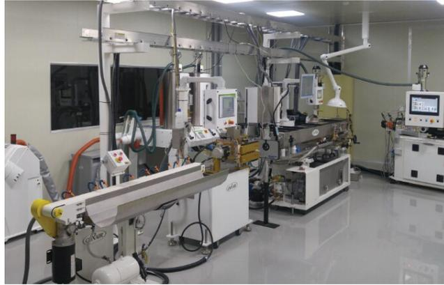
**Figure 1.** Medical multi-lumen tubing extrusion system.
