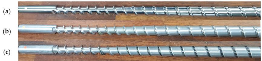
**Figure 5.** Three screws used in the screw wear experiments: (a) wear level 1: intact; (b) wear level 2: moderate wear; and (c) wear level 3: severe wear.
