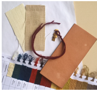
Figure 3. Photography of the examined test samples. Two different types of woven fabrics made of linen and hemp are shown in the top left corner. On the right side lies a piece of cowhide leather. Between the cloth and the leather, a replicated bird fibula is placed. The bottom row shows strands of dyed wool.
