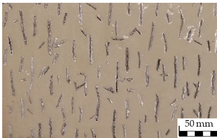
Figure 6. Recycled rCF yarn pieces as reinforcement in concrete.
